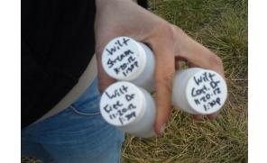
Grab Samples were taken from inside the controlled and conventional drainage structures and were analyzed for dissolved nitrate (NO<sub>3</sub><sup>-</sup>) and dissolved phosphate (PO<sub>4</sub><sup>3-</sup>)
