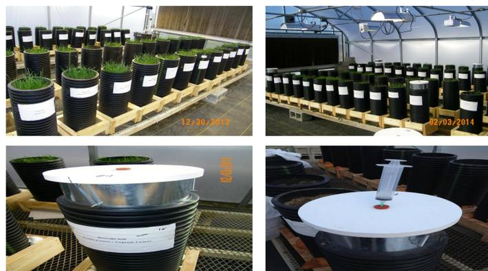
Figure 2. Greenhouse experiment and greenhouse gas chambers inserted in soil columns.
