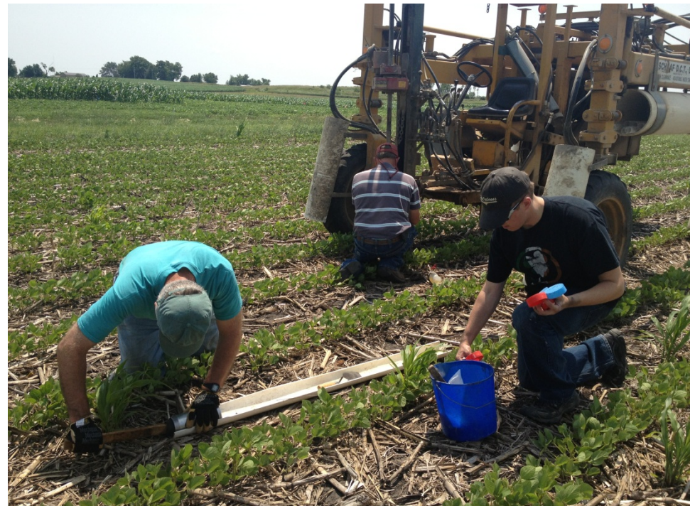
Intact soil core sampling for water retention analysis
