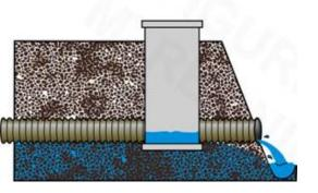
The outlet is lowered a few weeks before planting and harvest to allow field to drain.
