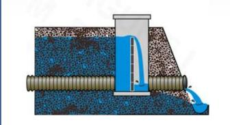
The outlet is raised after harvest to reduce nitrate delivery.
